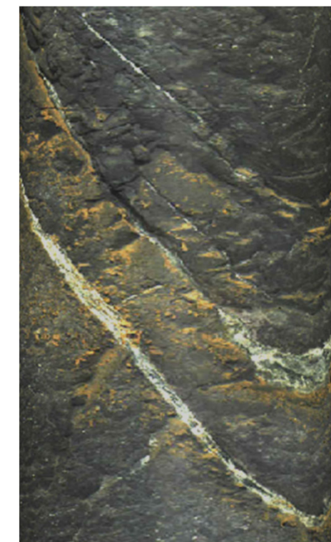
Steeply-Dipping Mineralized Fractures @ 65' to 67'
